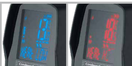
Illuminated LC display with colour alarm function
